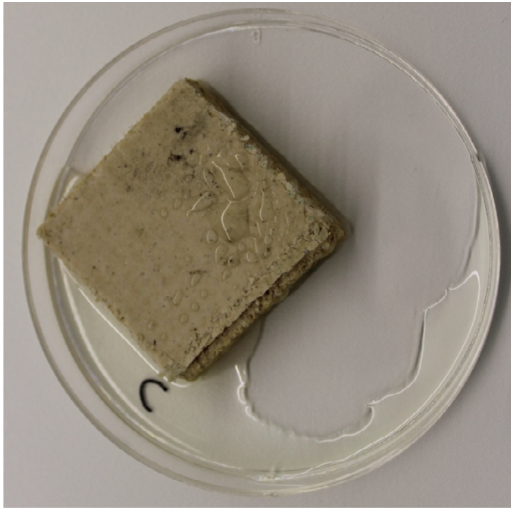
Figure 4-4- Evidence of leachate on sample C
