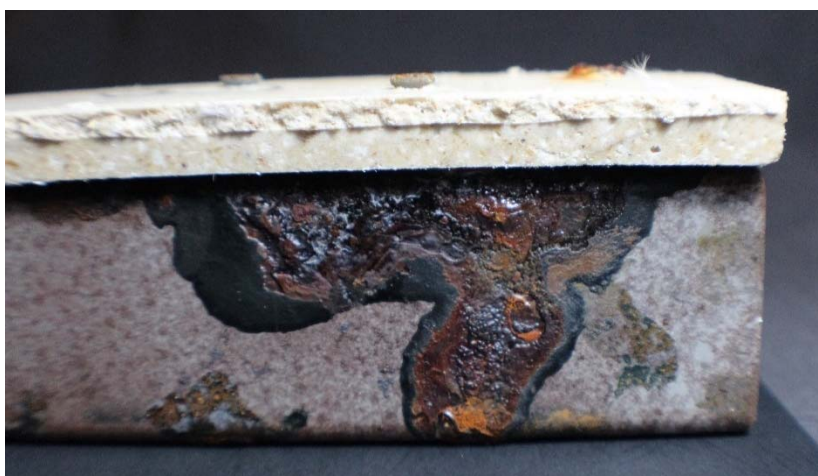
Figure 4-20-Corrosion of steel section due to leachate
