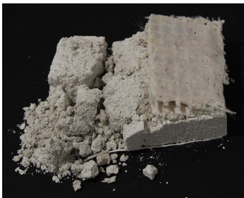
Figure 4-14- MgO sample C after 24 hours at 500°C
